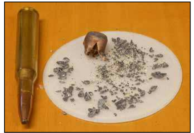
Lead bullets can fragment into hundreds of tiny pieces. Photo courtesy of HuntingWithNonLead.org
